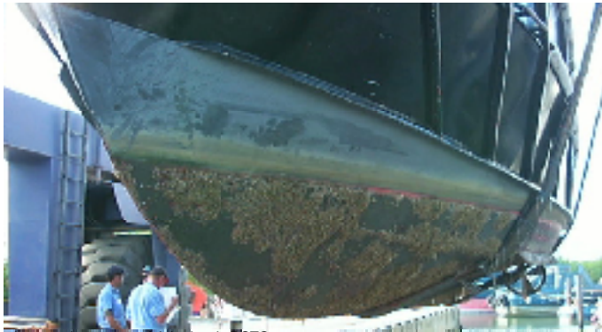
photograph courtesy of John Lewis DSTO
